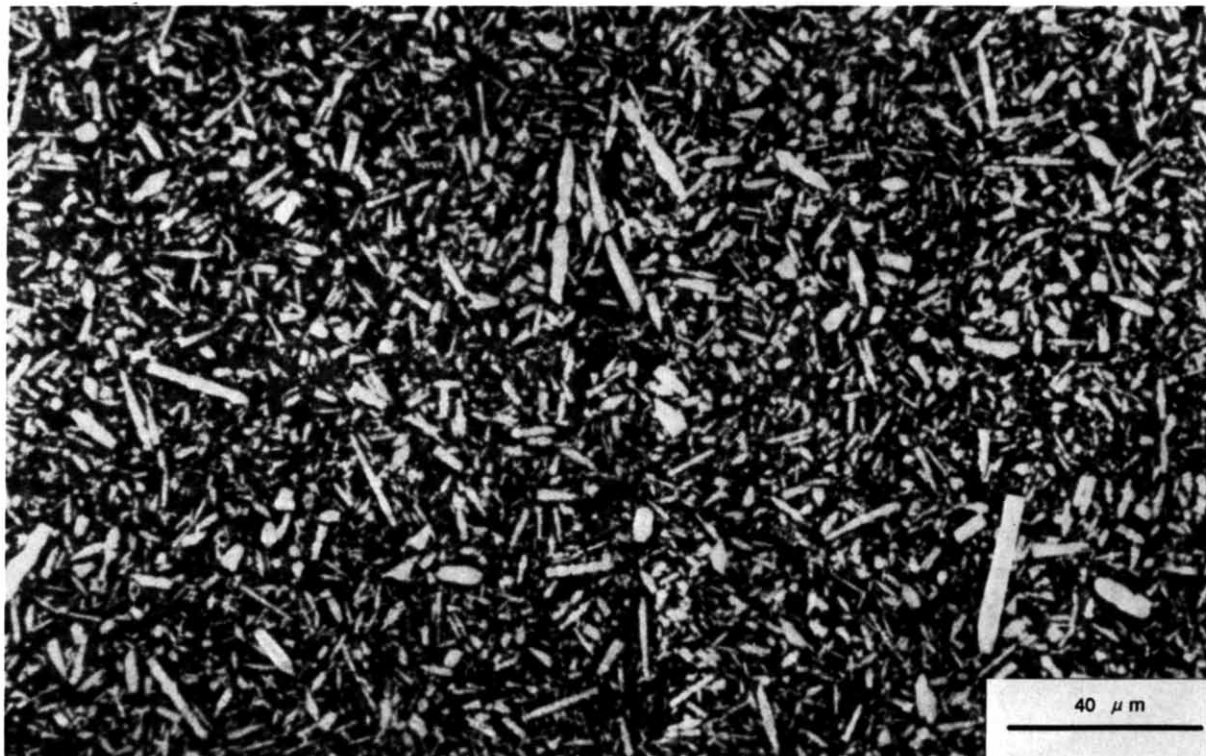
Fig. 4. Cross-section of a hot-pressed alumina/silicon carbide whisker composite with about 40 vol.% reduced aspect ratio whiskers. Note the absence of whisker clusters or whisker-depleted regions.
